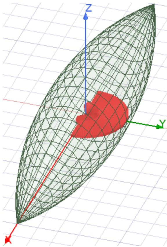
This setup will solve for the response due to incident plane waves at  $\theta = 90^\circ$  and for 61 values between  $\varphi = 0^\circ$  and  $\varphi = 180^\circ$ , inclusively. The polarization is  $\varphi$ -directed, so we will be solving for the HH monostatic RCS.
