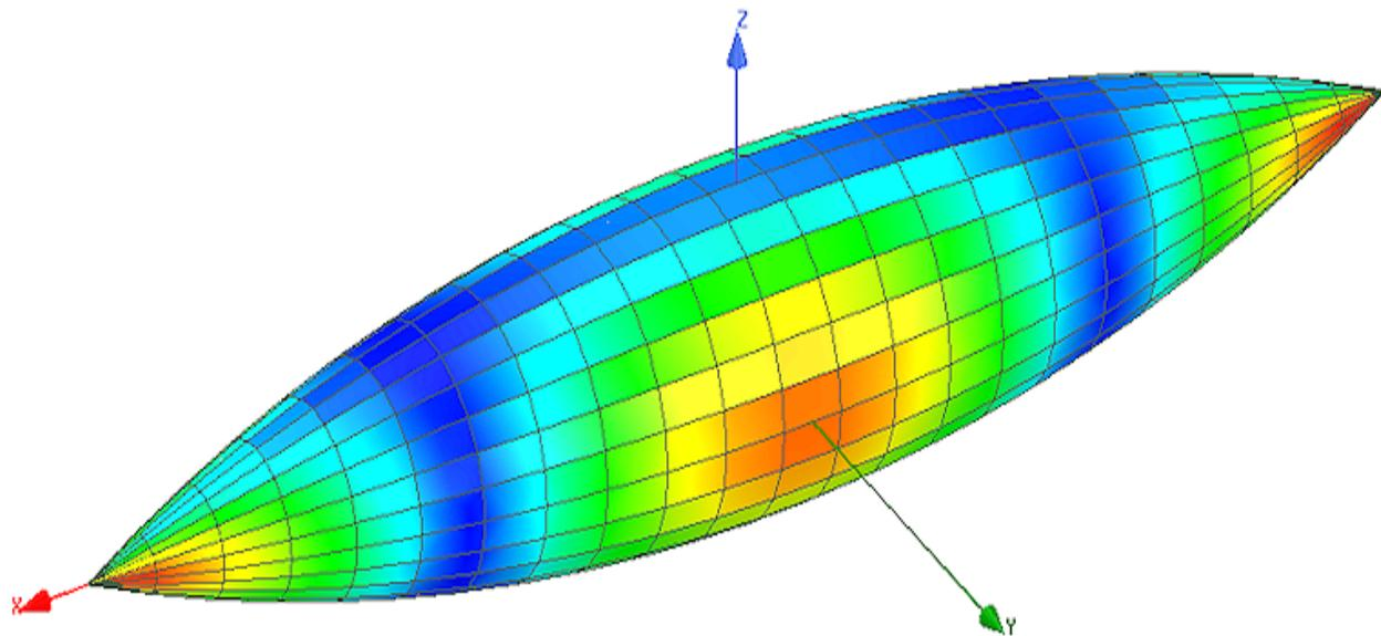
We will look at the scattering from a conducting ogive with a length of 10" and a half angle of 22.6° (0.3948 radians). The ogive lies with its axis along the global X axis. The equation that defines this model is:
