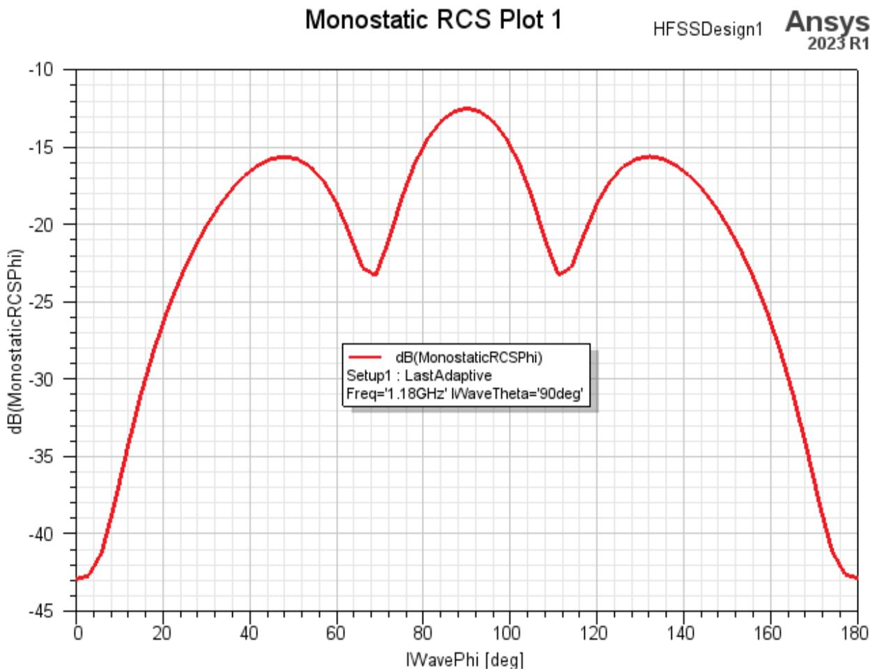
This plot is the HH monostatic RCS pattern for the standard ogive at 1.18GHz.
